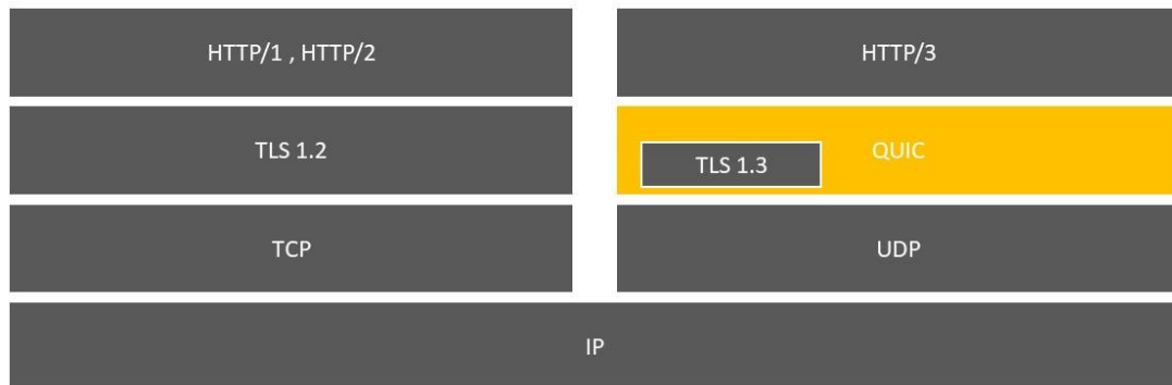
Fig. 3. Internet Stacks: HTTP/1 & HTTP/2 vs HTTP/3
